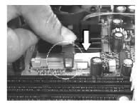
Step7: Finally, attach the fan cable to the CPU fan header FCPU.
