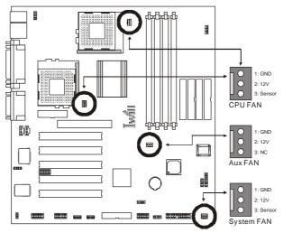
J39: CPU 0 Fan header (J39) J40: CPU 1 Fan header
