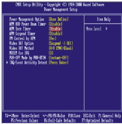
Each power-saving mode has a respective timer. The value of the timer can be assigned or reloaded and it will count down to zero. When the timer equals to zero, the system will be forced into the related suspend or power-saving mode. If any predefined signal or event is detected during the timer counting period, the timer restarts automatically.
