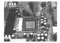
Step 5: Attach the heatsink onto the CPU.
