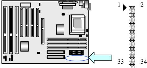
The FDC sub-system can control three types of floppy drives (1.2, 1.44 and 2.88MB) or compatible tape drives. The connection to the floppy drive is via a header (J19). The floppy disk interface includes 48mA drivers and inputs on the drive interface.
