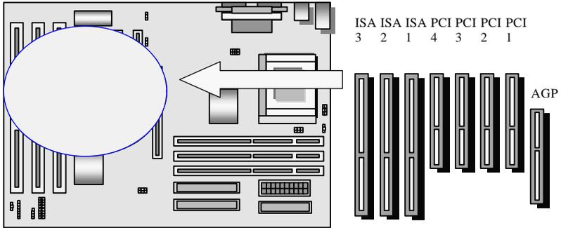
This motherboard contains 8 expansion slots onboard. Three 16-bit ISA Bus, four 32-bit PCI expansion slots and one 32-bit AGP slot as shown above.
