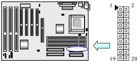
This connector supports a standard ATX power supply. When connecting, make sure the lock key matches the hook attached on a power supply cable. The power cord should be unplugged when you connect it.
