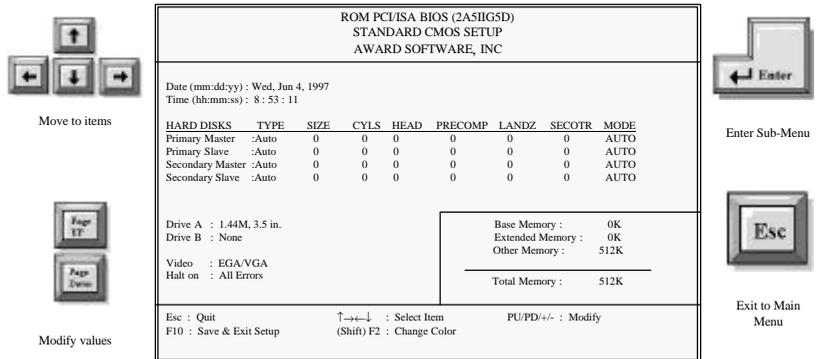
Figure 2: Standard CMOS setup
