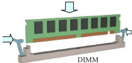
Be careful not to misfit the DIMM Module into DIMM sockets in wrong direction. This module can be inserted into DIMM socket only one way. Please note the “▲” for pin 1 location. To release the memory module, push both latches down and carefully rock the module forward and backward while slowly lifting it upward.
