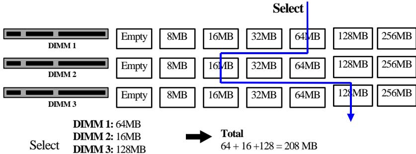
To select 1 out of 7 items (empty, 8MB, 16MB, 32MB, 64MB, 128MB, 256MB) in DIMM3.
