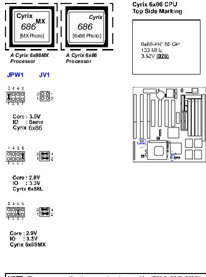
NOTE : The same specifications may be observed for IBM 6x86/6x86MX CPUs. Only Cyrix Rev 2.7 or later is supported on this mainboard. Bootup screen will show 6x86-P166+ with the Cyrix 166+ installed on this mainboard.
