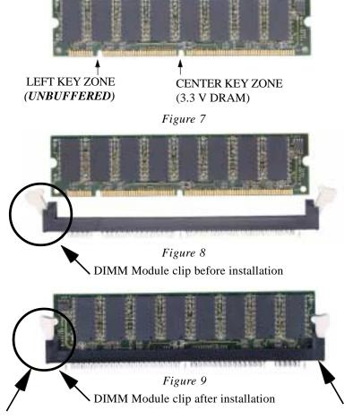
To remove the DIMM module simply press down both of the white clips on either side and the module will be released from the socket.
