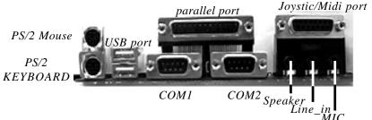
Figure 3: I/O back panel layout
