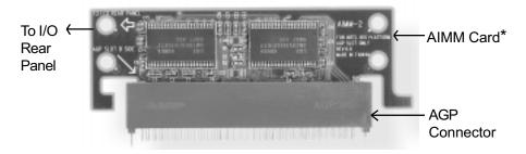
Note: The AIMM card for Intel 815 chipset M.B's AGP slot only. \* : The AIMM Card (optional)
