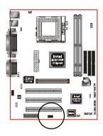
**USB2:** USB port header pins for share with two USB ports.
