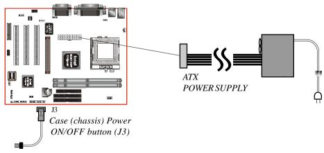
Figure 4: Simple ATX Power ON/OFF Controller
