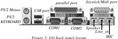
Figure 3: I/O back panel layout
