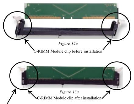
To remove the C-RIMM module simply press down both of the white clips on either side and the module will be released from the socket.
