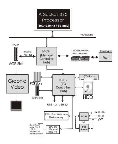
Figure 5: System Block Diagram
