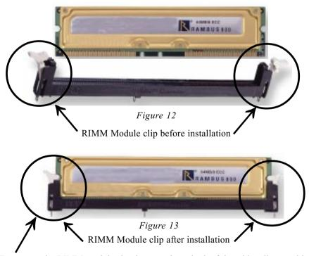
To remove the RIMM module simply press down both of the white clips on either side and the module will be released from the socket.
