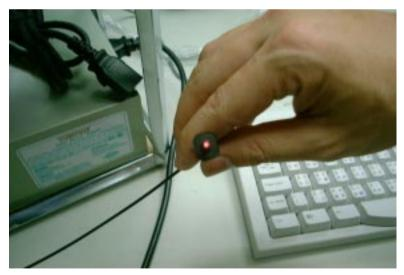
Please note that signal beam may cause severe damage to the eyes. For your safety, please point the output end to a piece of white paper to check if thebeam is in function.
