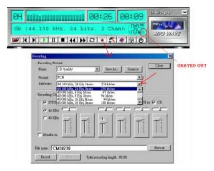
24-bit audio can only be applied to SPDIF IN/OUT mode; it does not apply to other modes such as the four channels or the analog. No sound will be heard while in playback, yet it can be recorded.
