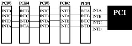
Figure 7: The Combination of PCI INT# lines
