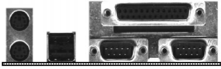
PS/2 Mouse USB 1 (Top) (Top) PS/2 Keyboard USB 0 (Bottom) (Bottom) Parallel Port (Top)
