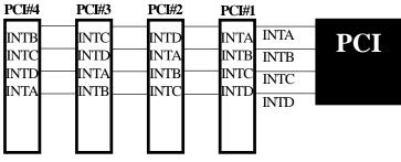
Figure 7: The Combination of PCI INT# lines
