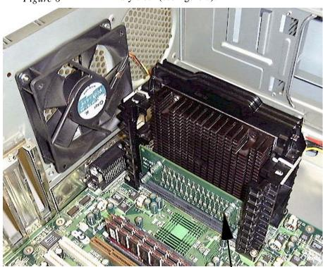
Figure 7. Completed assembly with 1 processor and terminator module.
