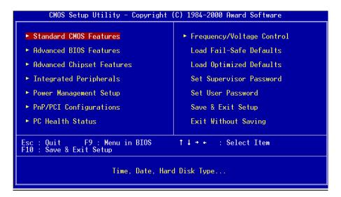
Figure 1: CMOS Setup Utility
