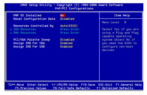
Figure 7: PCI Configuration Setup
