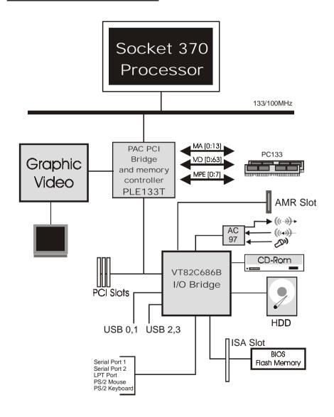
Figure 5: System Block Diagram
