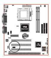
**USB2:** USB port header pins for share with two USB ports.
