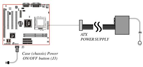
Figure 4: Simple ATX Power ON/OFF Controller
