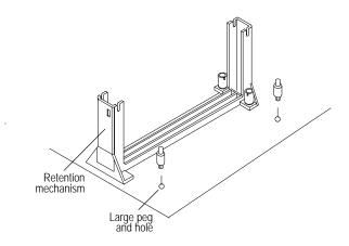
2. Slide a black plastic heatsink support onto each end of the fan heatsink, making sure that the hole and clip are on the outside edge of the support. (If the supports are reversed, the holes will not line up with the pegs on the system board). Slide each heatsink support toward the center of the processor until the support is seated in the outside groove in the fan housing.
