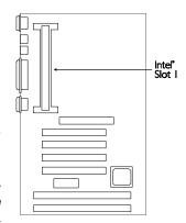
(for floppy drive, hard drive, CD-ROM, etc.) must be routed clear of the processor and its airspace. Otherwise, the processor will overheat and damage the processor and the system board.
