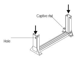
5. Tighten the captive nuts to stabilize the Retention Mechanism.
