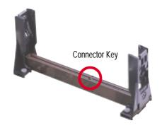
2. Push down firmly but gently the SECC2/SECC/SEPP into the URM until it snaps into place.
