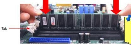
**Note:** The tabs of the DIMM slot will close-up to hold the DIMM in place when the DIMM touches the slot's bottom.
