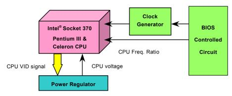
(Automatically generates CPU voltage)
