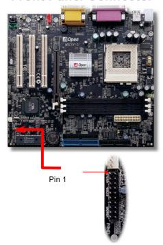
Attach the power LED, speaker, Power and reset switch connectors to the corresponding pins. If you enable "Suspend Mode" item in BIOS Setup, the ACPI & Power LED will keep flashing while the system is in suspend mode.
