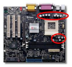
The power circuit of the CPU core voltage must be checked to ensure system stability for high speed CPUs (such as the new
