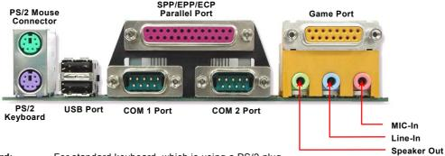
**PS/2 Keyboard:** For standard keyboard, which is using a PS/2 plug.
