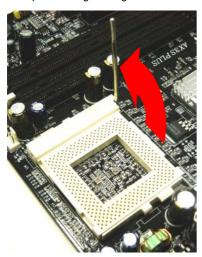
Locate Pin 1 in the socket and look for a black dot or cut edge on the CPU upper interface. Match Pin 1 and cut edge, then insert the CPU into the socket.
