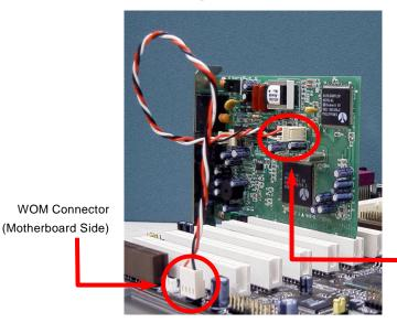
With the help of the ATX soft power On/Off, it is possible to have a system totally power off, and wakeup to automatically answer a phone call as an answering machine or to send/receive a fax. You may identify whether or not your system is in true power off mode by checking to see if the fan of your power supply is off. Both an external box modem and an internal modem card can be used to support Modem Wake Up, but if you use an external modem, you have to leave your box modem on.
