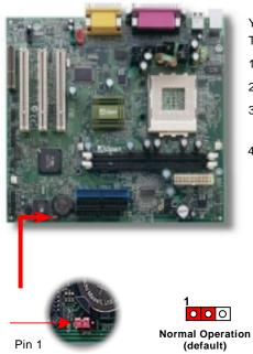
You can clear CMOS to restore system default setting. To clear the CMOS, follow the procedure below.
