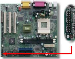
Attach power LED, EMPI, speaker, power and reset switch connectors to the corresponding pins. If you enable "<u>Suspend</u> <u>Mode</u>" item in BIOS Setup, the ACPI & Power LED will keep flashing while the system is in suspend mode.
