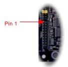
Attach the power LED, EMPI, speaker, power and reset switch connectors to the corresponding pins. If you enable "Suspend Mode" item in BIOS Setup, the ACPI & Power LED will keep flashing while the system is in suspend mode.
