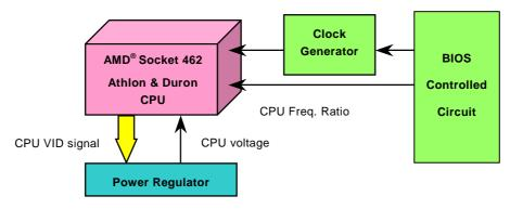
(Automatically generates CPU voltage)
