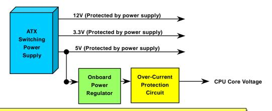
**Note:** Although we have implemented protection circuit, try to prevent any human operating mistake. There is still certain risk that CPU, memory, HDD, and add-on cards installed on this motherboard may be damaged because of component failure, human operating error or other unknown reasons. **AOpen cannot guarantee the protection circuit will always work perfectly.**
