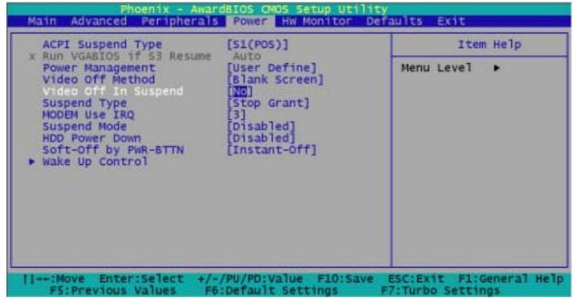
The Power Management Setup Menu allows you to configure your system to utilize energy conservation and power up/power down features.
