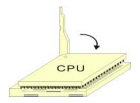
3. Press the lever down. Then Put the CPU fan on the CPU socket and clasp it with the socket. When the CPU fan is fixed to the CPU socket, put the fan's power port into the CPUFAN. After finishing all these steps, the CPU is ready for use.
