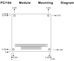
Step5 Secure the PC/104 module onto the CPU card using the four mounting spacers and srews.
