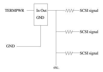
Assuming that the TERMPWR voltage doesn't drop below the desired termination voltage (plus the regulator's minimum drop), the SCSI signals will always be terminated to the correct voltage level.
