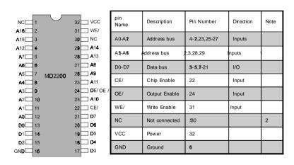
Note 1: Pins A13 through A16 are not used by the MD2200. They are kept for socket backward compatibility with ED 1100 (DiskOnChip 1000)
