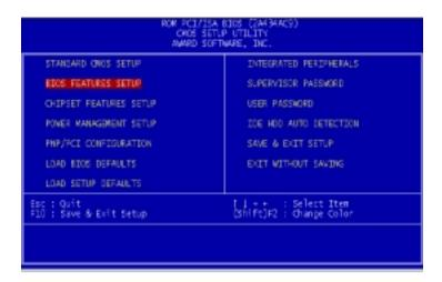
By choosing the BIOS FEATURES SETUP option from the INITIAL SETUP SCREEN menu, the screen below is displayed.
