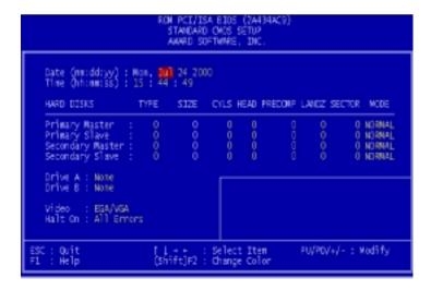
This standard setup menu allows users to configure system components such as the date, time, hard disk drive, floppy drive, display, and memory. Online help for each field can be accessed by pressing F1.
