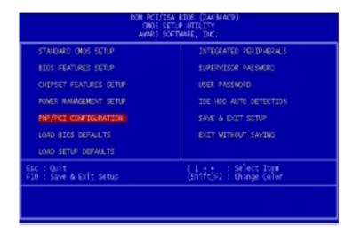
By choosing the PNP/PCI CONFIGURATION SETUP option from the initial SETUP SCREEN menu, the screen below is displayed.
