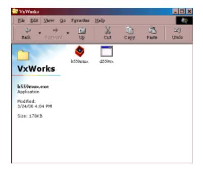
After installing the provided CD in the CD-ROM player this widow will appear. Double click on the *b559mus* icon to proceed with the installation. The file name for ethernet installation is 82559ER, in the 82559erdrivers16.zip.
