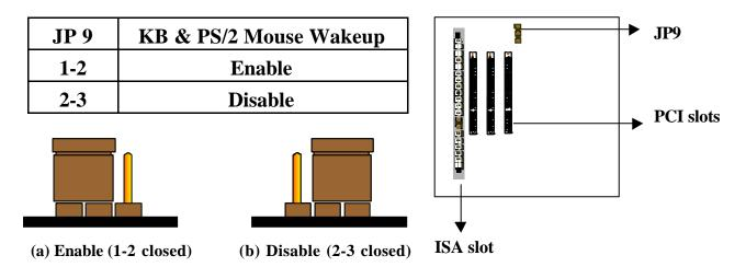
The default Power On function is "Button Only". That means, we can only turn our computer on and off by pressing the "Power Button". If we want to enable KB & PS/2 Mouse Power On function, we first have to set JP9 to Pin 1-2 closed, and then go to "Power On Function" in "Integrated Peripherals" of Award BIOS Setup. At the line "Power On Function", we can press "Page Up" or Page Down" to make the following selections:
