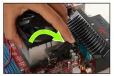
**7.** Turn the cam lever to lock into the retention frame.
