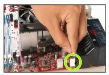
8. Attach the four-pin power plug from the heatsink and fan assembly to the CPU FAN connector.
