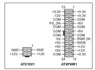
**Note:** It is recommended to connect to a power with 350W, 20A +5VDC capacity at least for heavily loaded system, and a 2A +5VSB capacity at least for supporting wake-up features.
