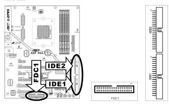
The FDC1 connector connects up to two floppy drives with a 34-wire, 2-connector floppy cable. Connect the single end at the longer length of ribbon cable to the FDC1 on the board, the two connectors on the other end to the floppy disk drives connector. Generally you need only one floppy disk drive in your system.
