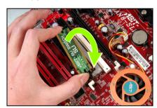
2. Flip the switchboard over to the side labeled with "SLI". Carefully insert the switchboard into the slot.
