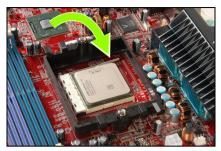
**3.** Lower the locking lever to the fully locked position.
