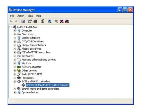
If an HPT370/HPT372 UDMA/ATA RAID Controller and HighPoint RCM Device item exists in the popup Device Manager window (see above), it indicates that the driver has been successfully installed.
