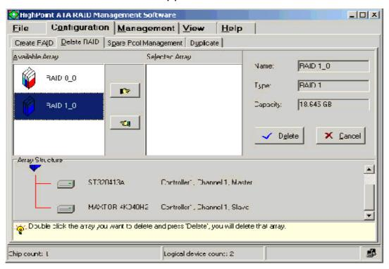
2. Select an array from the **Available Array** list box and click the " right hand" button to add it to the **Selected Array** list
