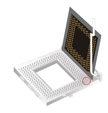
Seat the processor in the socket completely and without forcing.
