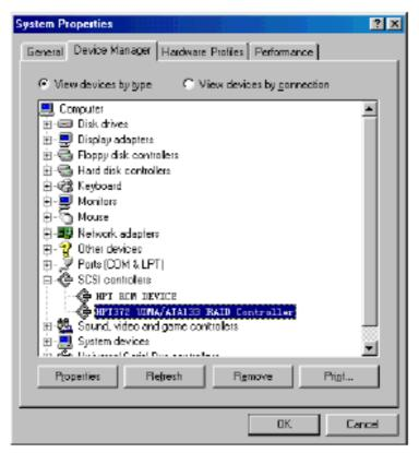
If you cannot find these two above-mentioned device items, or there are ? or ! on device icon, it indicates that the driver has not been correctly installed and needs reinstallation.
