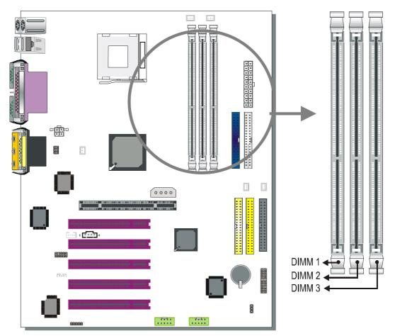
Your board comes with three DIMM sockets, Directly supports one DDR SDRAM channel, 64b wide, providing support max of 3 Double-Sided DIMMs with unbuffered DDR 266. *The largest memory capacity possible is 3GB.* On this motherboard, DRAM speed can be set independent from the CPU front side bus speed. Depending on the DRAM clock speed setting in the BIOS setup.
