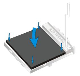
4. Then close the socket handle to secure the CPU in place.
