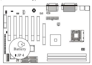
Normally JP4 will be in the 1-2 position, this will connect the battery to the southbridge of the chipset which contains the CMOS memory. If JP4 is temporarily set to 2-3 this will
