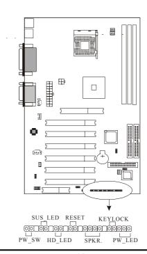
**PW\_SW** with a 2-pin Berg strip on case front panel indicates the current power status of system. It is used to connect to the Power Button on the front panel of the case (if there is).
