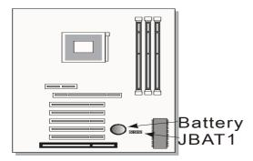
Normally JBAT1 will be in the 1-2 position, this will connect the battery to the southbridge of the chipset which contains the CMOS memory. If JBAT1 is temporarily set to 2-3 this will interrupt the battery electricity flow, and the CMOS memory will be erased, this will however only work if the power supply is not switched on. Now at the next reboot the BIOS will automatically load the CMOS default values.
