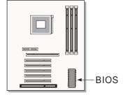
The BIOS IC is inserted in an IC socket, which means that it can be removed and exchanged for another IC if necessary.
