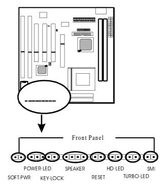
**SOFT-PWR** is ATX Soft-PWR with 2 pins. SOFT-PWR is for ATX power supply only.
