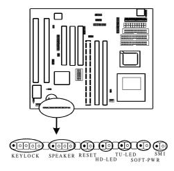
**KEYLOCK** is a 5-pin connector. It is used to connect the key lock on the case front panel (if there is). Keyboard may be disconnected with the system through this function. Set to "on" to disconnect the connector with the system and "off" for normal status.
