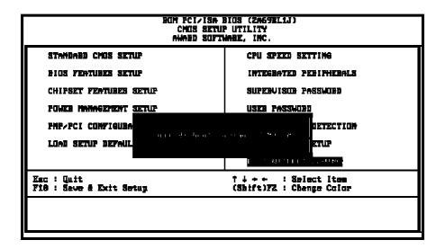
The "Quit Without Saving" option will bring you back to normal boot up procedure without saving any data into CMOS RAM. All of the old data in the CMOS will not be destroyed.
