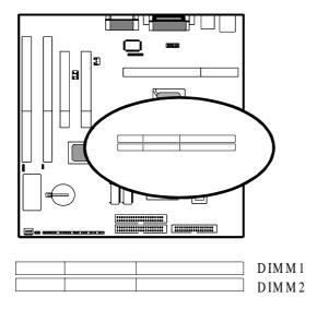
Insert the module as shown. Due to different number of pins on either side of the breaks, the module will only fit in the orientation as shown.
