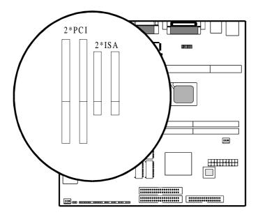
**There are** two standard PCI slots on board. 133MB/s data transfer rate on PCI bus can be compared to 33MB/s on EISA bus or 8MB/s on ISA bus. Synchronous operation CPU to PCI interface makes good graphic performance.
