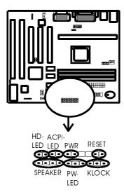
**HD-LED** (Hard Disk activity LED connector) is a 2-pin keyed Berg strip. It is used to connect to front panel Hard Disk LED.
