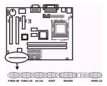
**POWER-LED** is a 3-pin connector. It is used to connect to the LED on the case front panel. The LED shows the status of the power.
