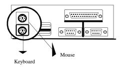
*The onboard PS/2 keyboard and mouse connector* is 6-pin Mini-Din connectors, marked as "KB" and "Mouse."
