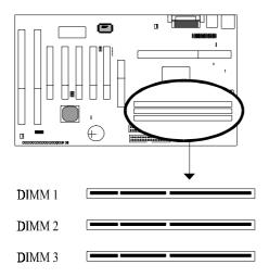
Insert the module as shown. Due to different number of pins on either side of the breaks, the module will only fit in the orientation as shown. There is no jumper setting for memory configuration.
