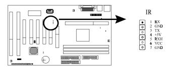
*IR connector* supports wireless infrared module. With this module and application software like LAPlink, or WIN95 Direct Cable Connection, user can transfer data to or from laptops, notebooks, PDA and printers. This connector supports **HPSIR**, **ASKIR**, and **Fast IR**.
