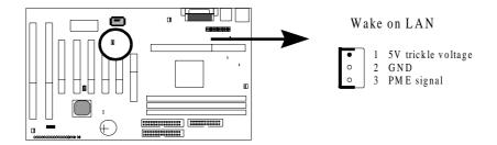
Wake on LAN, marked as "WOL," is a 3-pin connector. To support this feature, a network card is required for the system. More than that, a network management software must be installed too.
