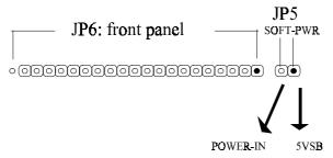
ATX soft-PWR switch connector is Soft-PWR with 2 pins.
