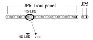
*Marked as "HD-LED*," Hard Disk activity LED connector is a 2-pin keyed Berg strip. It is used to connect to front panel Hard Disk LED.
