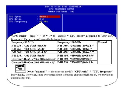
Since this is jumperless designed, there is no jumper setting to adjust CPU speed. The user only needs to set speed in BIOS. Please enter BIOS & find "CPU speed" item under "Chipset features setup" and set as above.
