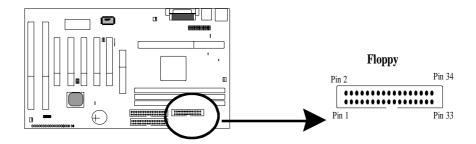
*Floppy interface connector* with 34 pins is used to attach the floppy drive cable.
