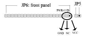
**Power LED** is 3-pin connector. It is used to connect to the LED on the case front panel. The LED shows the status of the power.
