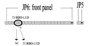
**Turbo LED** with a 2-pin Berg strip on front panel indicates the current speed status of system. It is used to connect to the Turbo Led on the front panel of the case (if there is).
