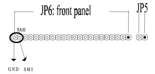
*SMI connector* is a 2-pin Berg strip, which is also called "green" or "sleep" connector. When SMI is turned from open to close and back to open, the system will enter sleep mode immediately. This function is to make sure power saving is working well. In PC system, it is used to connect to the push button SMI switch located on the case's front panel (if there is). The system can be forced to power saving mode by pressing the SMI switch.
