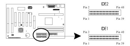
*IDE 1/ IDE 2* both have 40 pins. There are 2 IDE connectors supported on this system board. IDE1 is primary channel, and IDE2 is secondary channel. Each channel supports 2 IDE devices, and 4 channels in total for this system board.
