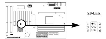
**SB-LINK** is used to attach any "PC/PCI" standard sound card like Creative AWE64D or Yamaha XG...for compatibility under DOS mode.
