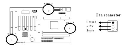
There are 3 fan connectors on this system board, and they are marked as "Fan 1," "Fan2," and "Fan3." Each fan connector has three pins.
