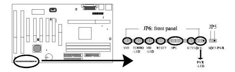
*Front panel* has connectors such as "SMI," "Turbo-LED," "HD-LED," "reset," "speaker," "keylock," and "power-LED." Please refer to details as below.
