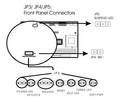
**POWER-** LED is a 3-pin connector. It is used to connect to the LED on the case front panel. The LED shows the status of the power.
