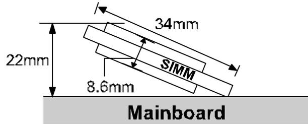
The SIMM installed cannot go beyond the dimensional requirements as shown in the above figure.
