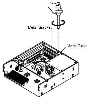
2. Firmly insert the add-on card on an available slot, in this example, the PCI slot.
