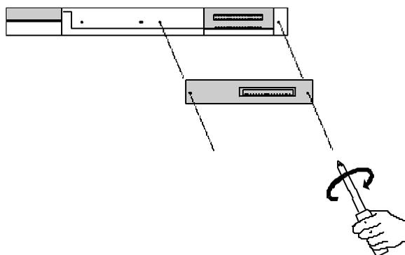
2. Attach the L-shaped metal bracket by matching the two screwholes of the metal bracket to the first and last screwholes of the group of four screwholes on the right underside portion of the slim CD-ROM drive and securing the two screws to it (see the following figure).
