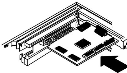
3. Insert the metal plate to affix the add-on card, and secure the screw on it.
