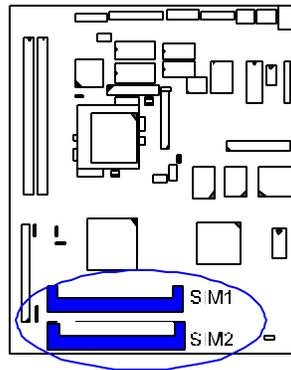
1. Locate the SIMM sockets on the mainboard.
