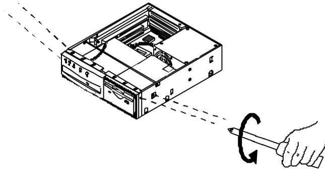
2. Pull the front chassis away from the main body about 10cm. Disconnect the ribbon cables and power wires of the FDD and CD-ROM drive.
