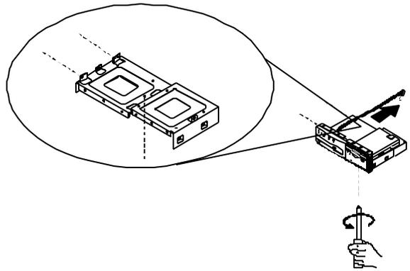
2. Remove the bracket on the side of the CD-ROM drive by loosening the two screws that affix it.
