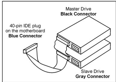
**NOTE:** Make sure to configure the “Master” and “Slave” relation before connecting two drives by one single ribbon cable. The red line on the ribbon cable must be aligned with pin-1 on both the IDE port and the hard-drive connector.
