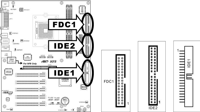
The FDC1 connector connects up to two floppy drives with a 34-wire, 2-connector floppy cable. Connect the single end at the longer length of ribbon cable to the FDC1 on the board, the two connectors on the other end to the floppy disk drives connector. Generally you need only one floppy disk drive in your system.
