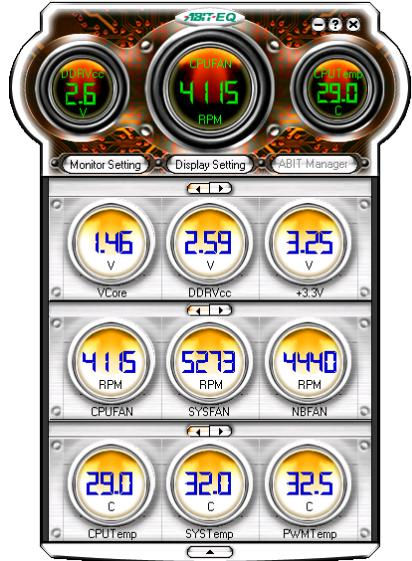
6. This screen appears. ABIT EQ shows you the status of Voltage, Fan Speed, and Temperature readings as well.
