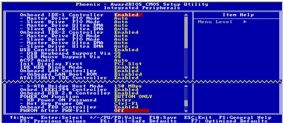
Figure 3-7. Integrated Peripherals Menu Screen
