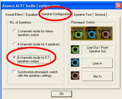
7. In this Speaker Configuration tab, check the “6 channels mode for 5.1 speakers output” box to enable 6-channel audio system.
