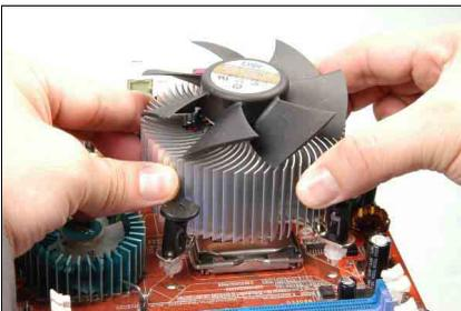
9. Place the heatsink and fan assembly onto the socket. Align the four fasteners toward the four mounting holes on the motherboard.
