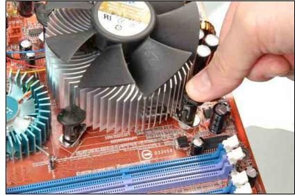
10. Press each of the four fasteners down into the mounting holes.
