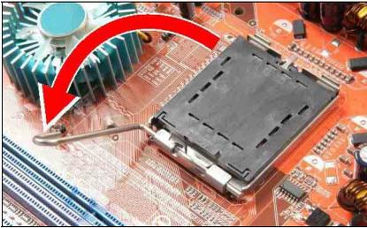
2. Rotate the lever to fully open position.
