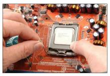
**7.** Lower the plate onto the CPU package. Engage the load lever while gently pressing down the load plate.
