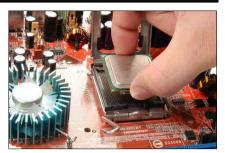
**4.** Use your right thumb and forefinger to grasp the CPU package. Be sure to grasp on the edge of the substrate, and face the Pin-1 indicator toward the bottom-left side. Aim at the socket and place the CPU package vertical down into the socket.
