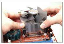
**9.** Place the heatsink and fan assembly onto the socket. Align the four fasteners toward the four mounting holes on the motherboard.
