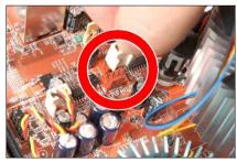
**12.** Attach the four-pin power plug from the heatsink and fan assembly to the CPU FAN connector.
