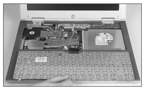
10 Disconnect the keyboard by lifting the keyboard connector using two fingers. Be careful to not touch or damage any other components.
