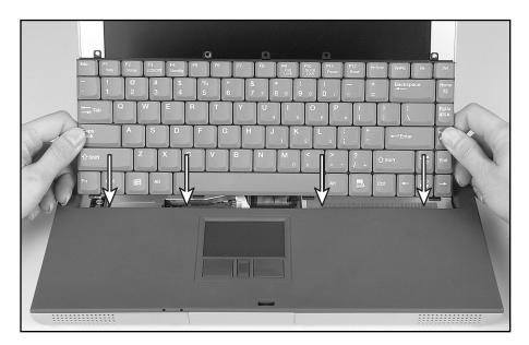
**5** Gently press the keyboard down until it is flat all the way across. The keyboard should easily fall into place. Be careful not to damage the LCD panel.
