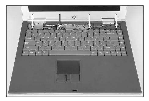
Slide the two tabs located on the left end of the bezel under the notebook frame.
