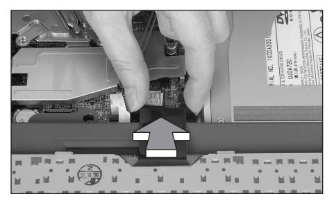
**3** Rotate the keyboard toward the LCD panel until the keyboard is almost face-up.
