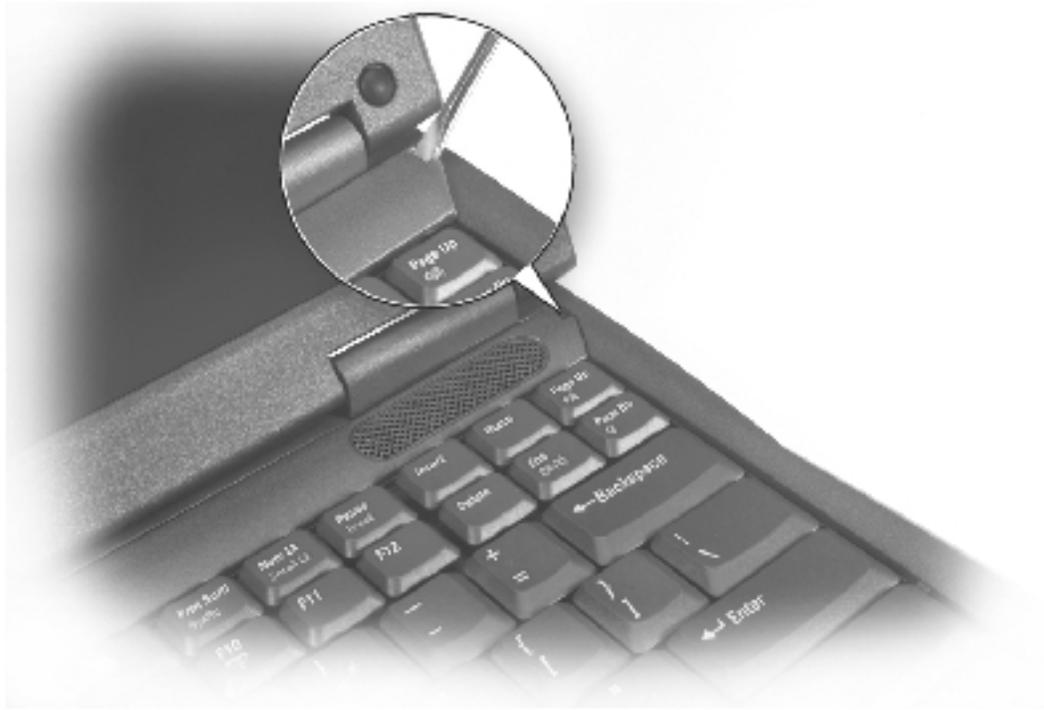
5. To release the keyboard from the palm rest, use a small, flat-blade screwdriver or plastic scribe to pry up the right edge of the keyboard near the blank key.
