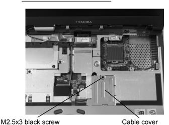
1. Remove **one M2.5x3 flat head screw** securing the cable cover.
