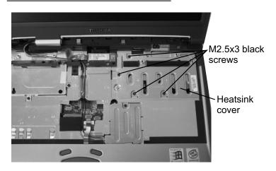
Remove four M2.5x3 brass screws securing the heatsink cover.
