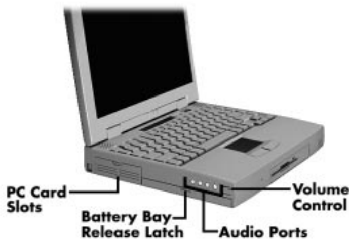
Figure 1-9 Left Side Features
