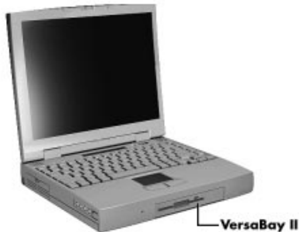
Figure 1-7 NEC VersaBay II Location
