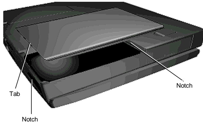
Figure Section 2-11 Battery Bay Cover Replacement
