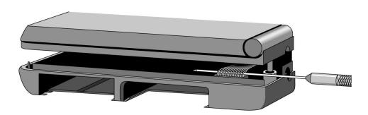
Figure 18 - Reconnecting Display Cable
