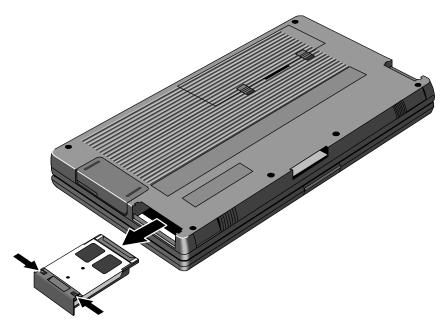
Figure 7 - Removing Card Slot Tray
