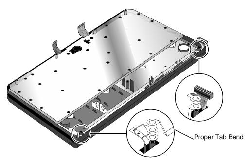
Figure 16 - Display Grounding Eyelets
