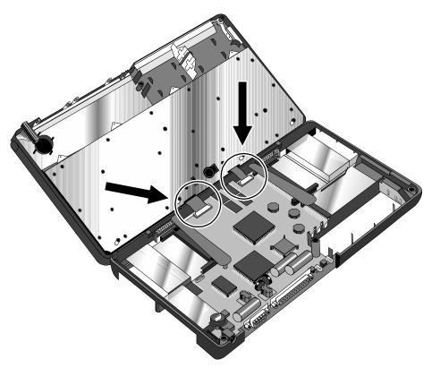
Figure 15 - Keyboard Flex Cables
