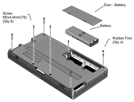
Figure 9 - Outer Bottom Case Components
