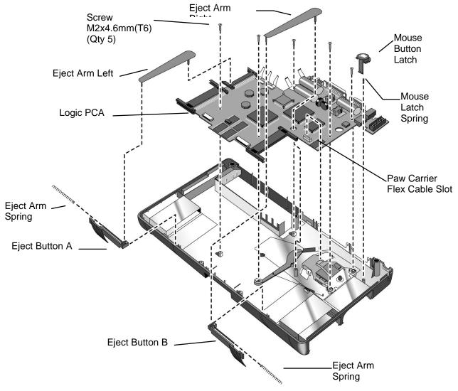
Figure 23 - Logic Board PCA Removal
