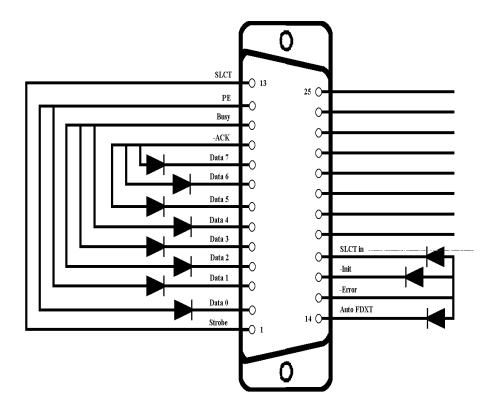
Figure 4 - Parallel Loop Back Connector
