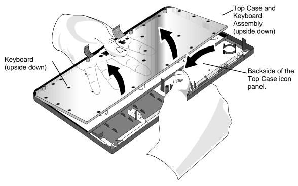
Figure - Keyboard Removal Hand Placement
