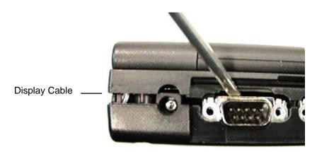
Figure 13 - I/O Port Prying Location
