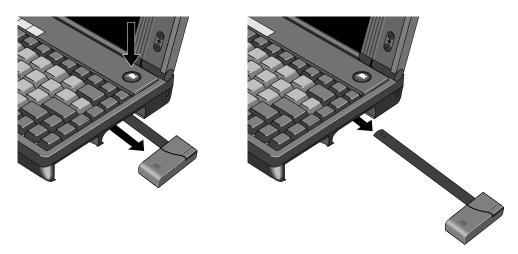
Figure 8 - Removing the Mouse
