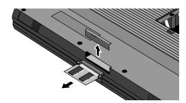
Figure 6 - Removing the Memory Module
