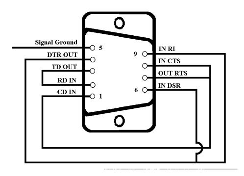
Figure 3 - Serial Loop Back Connector
