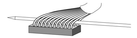
Figure 17 - Display Cable Probe Position
