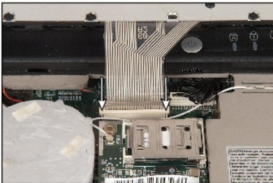
5. Press down on the keyboard connector using two fingers. This locks the keyboard cable into the keyboard connector.
