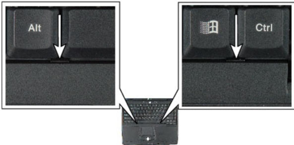
9. Insert the small flat blade screwdriver next to these tabs and pry the keyboard up. Be careful to pry up on the keyboard base and not on one of the keys.
