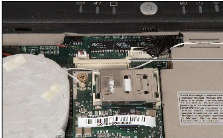
4. Slide the end of the keyboard cable into the keyboard connector.
