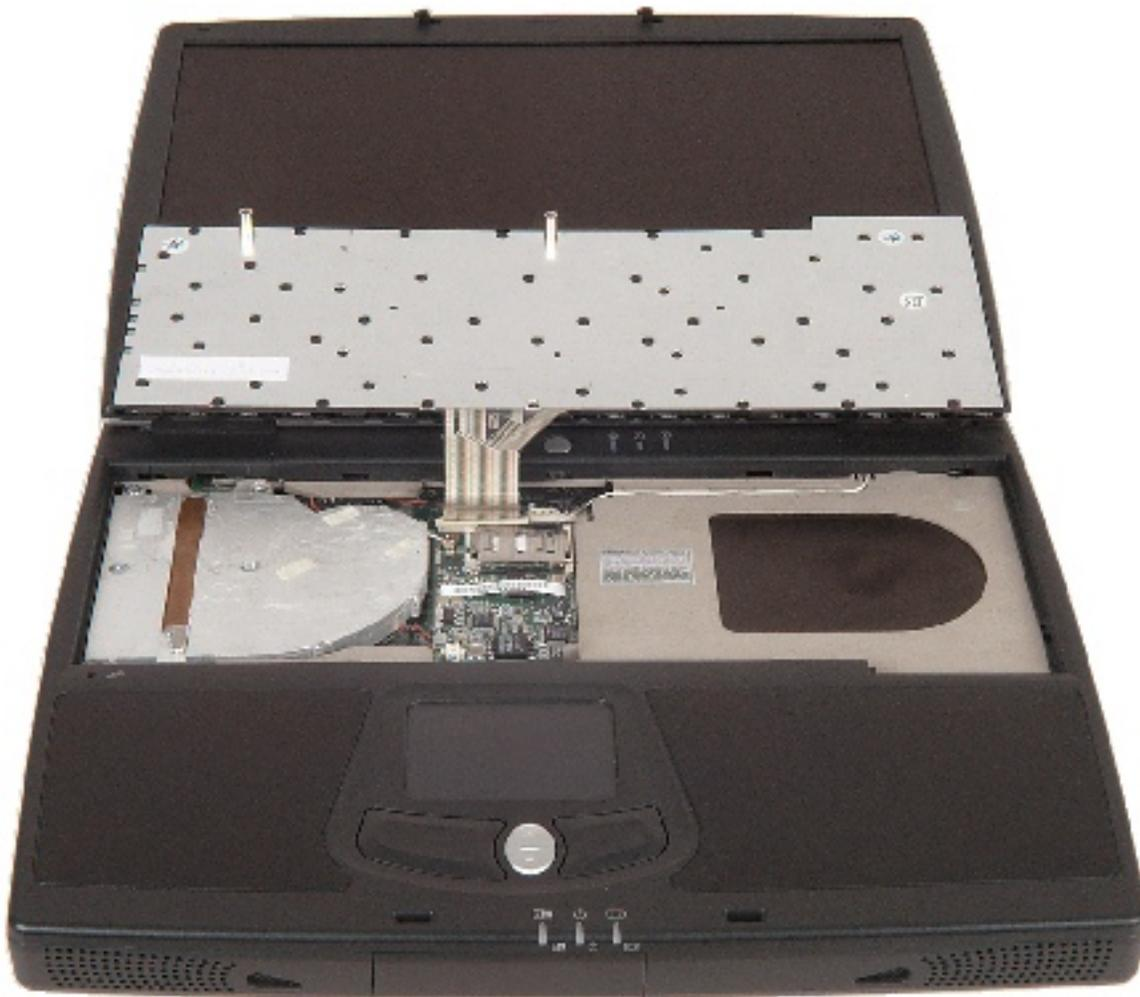
13. Disconnect the keyboard by pulling up on the plastic keyboard connector using two fingers. Once the keyboard connector is in the raised position, gently pull the keyboard cable out of the connector. Be careful to not touch or damage any other components.
