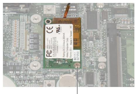
**26** Turn the system board over and remove the screw that secures the modem to the system board.
