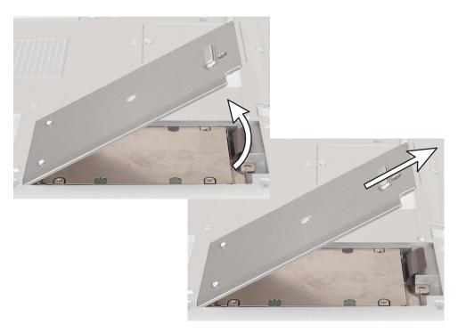
**6** Lift the screw side of the cover upward, then slide the cover out.
