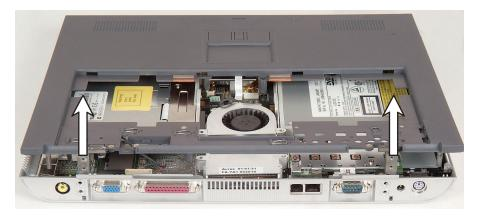
**16** While holding the palm rest assembly up, unplug the fan cable. Make sure that you unplug the connector by grasping the connector, not the cable.
