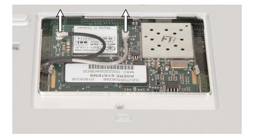
**8** Move the antenna wires out of the way, then press outward on the clips at both sides of the module until the module tilts upward.
