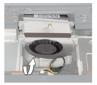
**15** Insert the new cooling assembly into the notebook, then tighten the four captive screws. Make sure that you tighten the screws in numerical order. Each screw hole has a numeral next to it.
