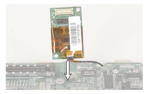
Install the modem into the new system board and turn the board over.
