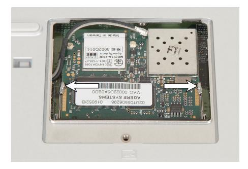
Pull the module out of the slot.
