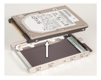
**8** Insert the new drive into the bracket so the screw holes line up, then replace the four screws that secure the drive to the bracket.
