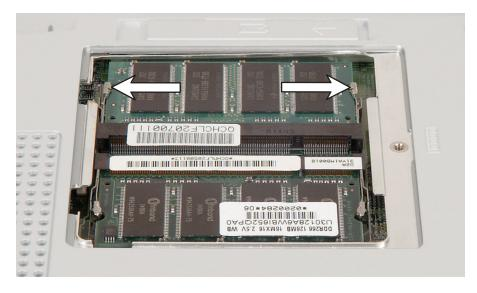
**8** Pull the memory module out of the slot.
