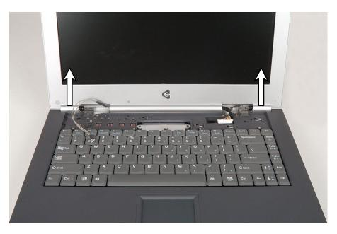
**13** Place the new LCD panel assembly onto the notebook, then replace the four (or six, depending on screen size) hinge screws. Make sure that you connect the LCD panel's ground cable to the left screw of the right hinge.
