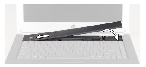
**10** Press down on the cover in several places until it clicks in place. The cover is correctly mounted when you can run you finger along the cover and find no loose spots. The cover should be flat all the way across.
