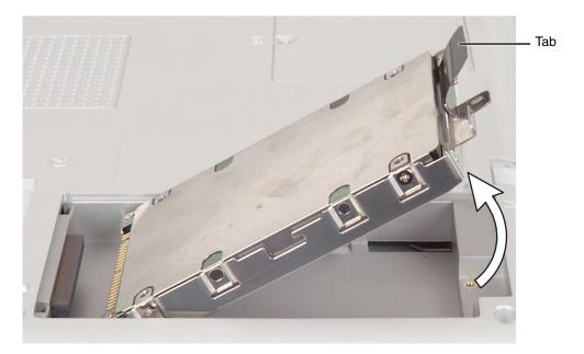
**9** Place the new hard drive kit into the drive bay, then slide the drive onto the connector.
