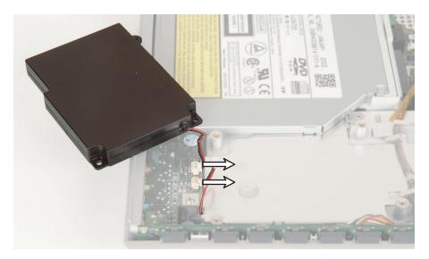
**14** Use a flat-blade screwdriver or non-marring tool to carefully pry open the metal tabs that secure the wires for the right speaker, then completely remove both speakers.
