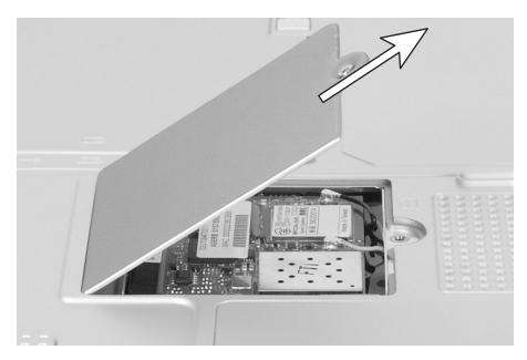
**7** Unplug the two antenna cables, noting which cable is attched to the connector labeled *Main* and which cable is attached to the connector labeled *Aux*.
