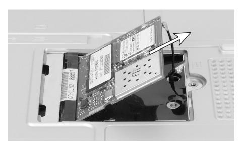
10 Hold the new card at a 30-degree angle and press it into the empty slot. This card is keyed so that it can only be inserted in one direction. If the card does not fit, make sure the notch in the card lines up with the tab in the card slot.
