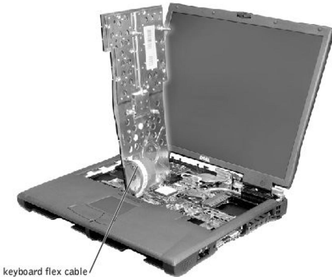
7. Disconnect the keyboard flex cable and lay the keyboard aside.
