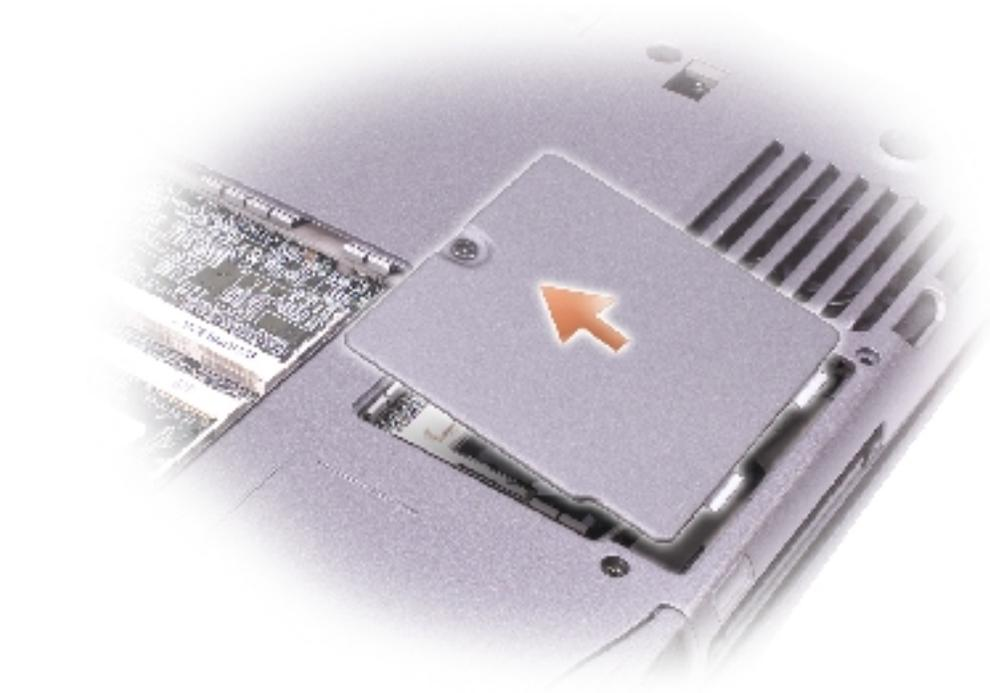
3. Place your finger under the cover at the indentation, lift up the cover, and slide the cover open.
